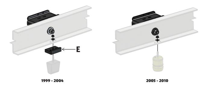
For 1999 to 2004 vehicles, the convoy clip must be removed between step 3 and step 4. When reinstalling the factory bump-stop in step 4 the Bump-Stop Spacer [ITEM E] will be incorporated to account for the removed convoy clip.
