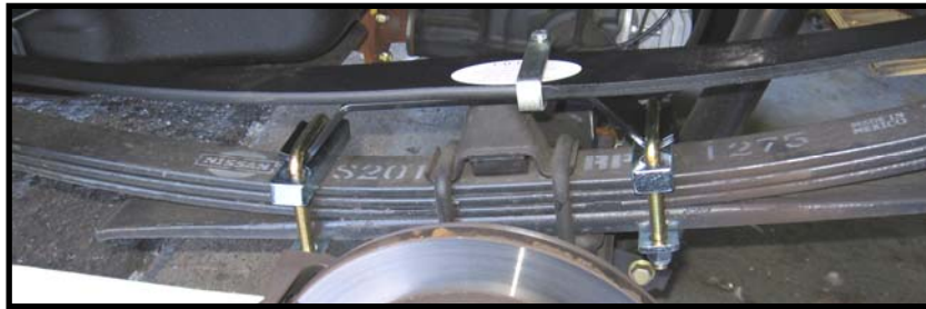
Special mounting kit with springs installed shown above – bump stop not show.
